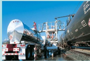
5. Ethanol unloaded from tank cars to tank trucks at rail terminals *
