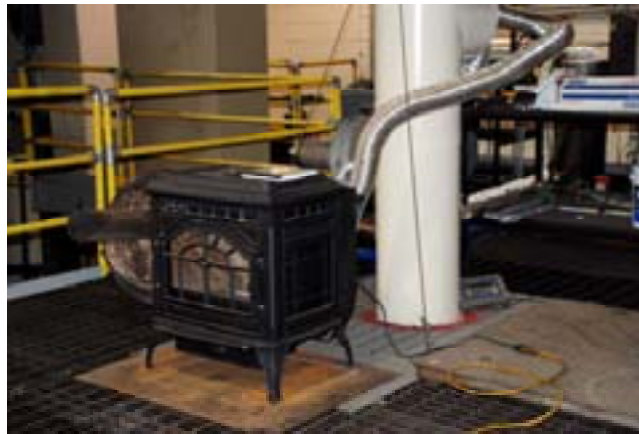
Residential pellet stove testing switchgrass pellets
