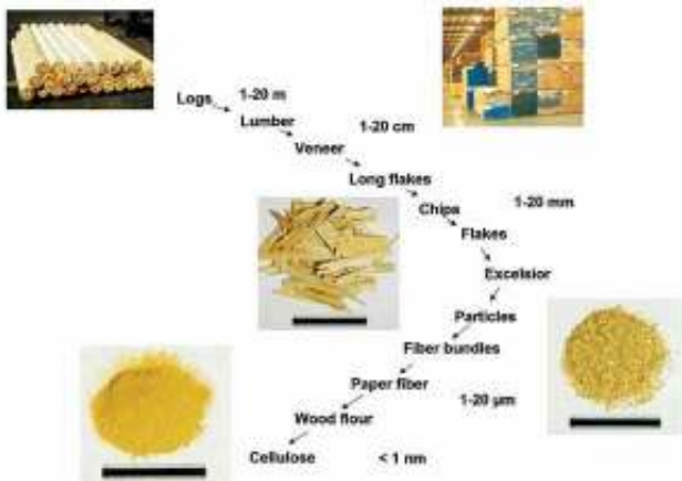
Ref: USDA Wood Handbook Figure 11-2. Basic wood elements, from largest to smallest (adapted from Kretschmann et al. 2007)
